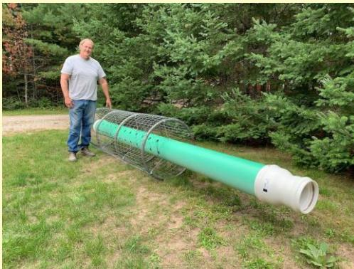
steel pipes formed into 30-inch diameter rings with ends welded together. I attach these to the plastic pipe through the use of threaded rods and pipe hanger brackets.
